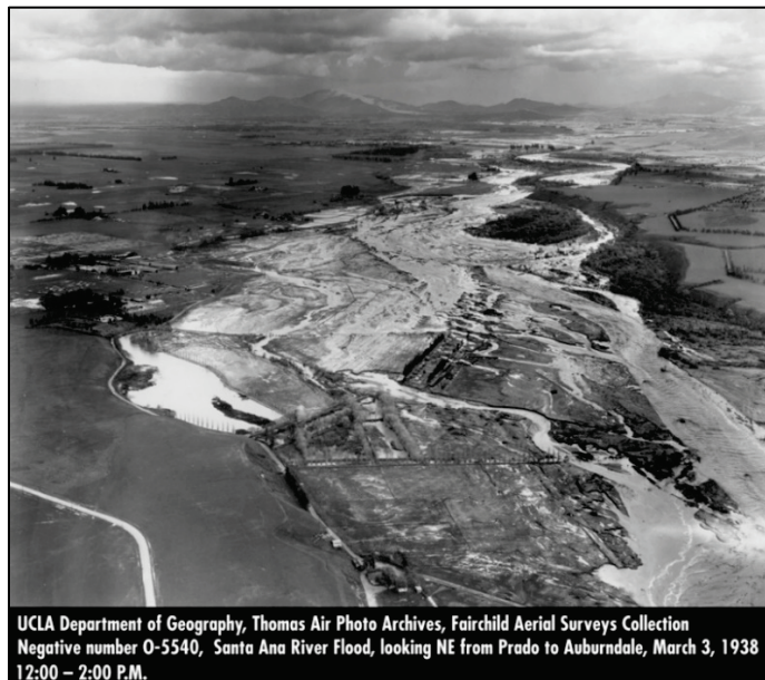
Figure 55. View looking upstream along Santa Ana River, flood of March 3, 1938, showing the braided pattern typical of southern California rivers crossing the coastal floodplain (With permission, University of California at Los Angeles Dept. of Geography).
