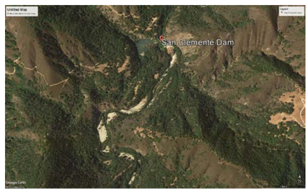
a. San Clemente Reservoir, CA – Photographs from Google Earth spanning two decades (1994 left and 2013 right) show the loss of reservoir storage capacity over time due to sedimentation.
