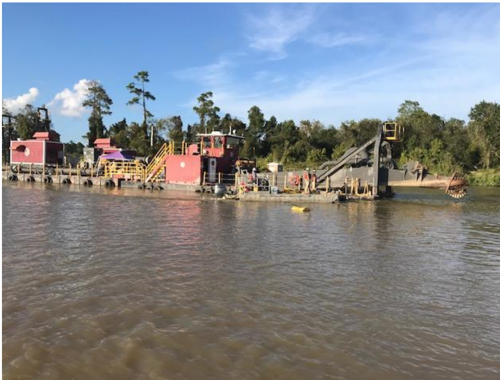
Figure 14 Example of Dredge with Ladder-Supported Submersible Pump
