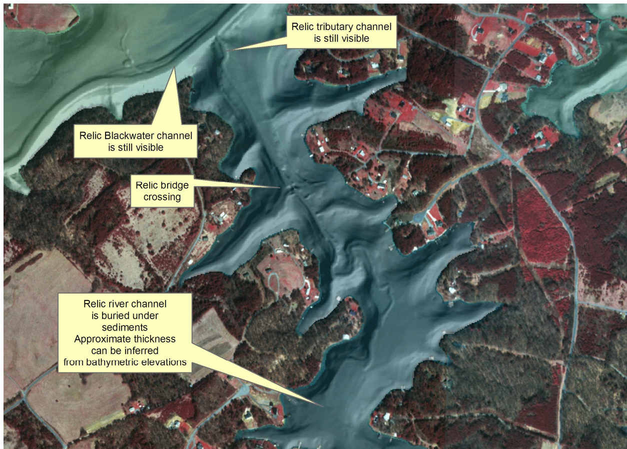
Figure 6: Example of bathymetric data illustrating relic features submerged beneath Smith Mountain Lake and obfuscation of relic channels by subaqueous reservoir sedimentation. Features minimally affected by sedimentation such as the lower river channels, an old bridge, and a road bed are still visible. Approximate depth of sediment accumulation may be estimated by the height of lost features as estimated from the bathymetric data. For example, the stream banks in this figure are approximately 2 feet high. Thus, there must be at least two feet of sedimentation at the point where the channel “disappears” beneath the sediment.
